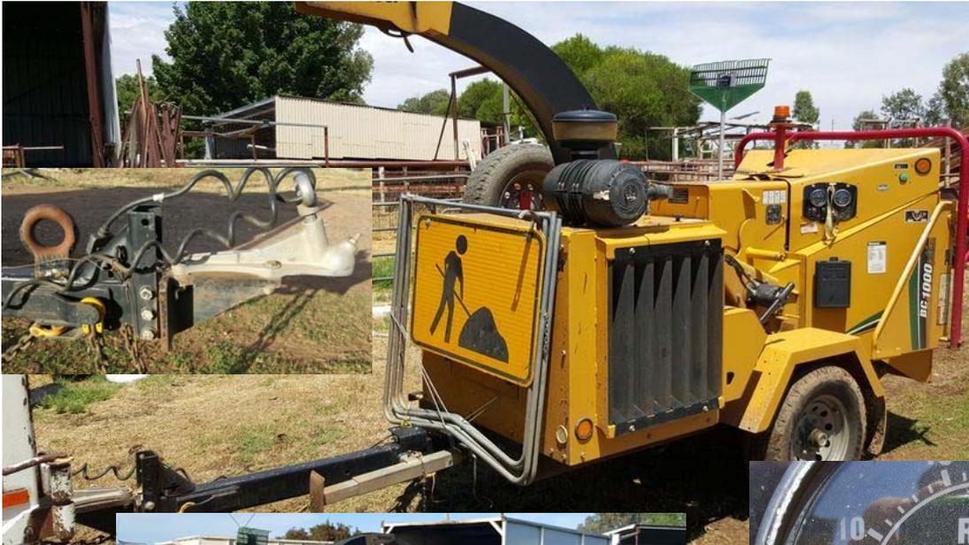
Chipper has 50 mm towball coupling but ring pull is included see it resting on the drawbar in insert photo.
